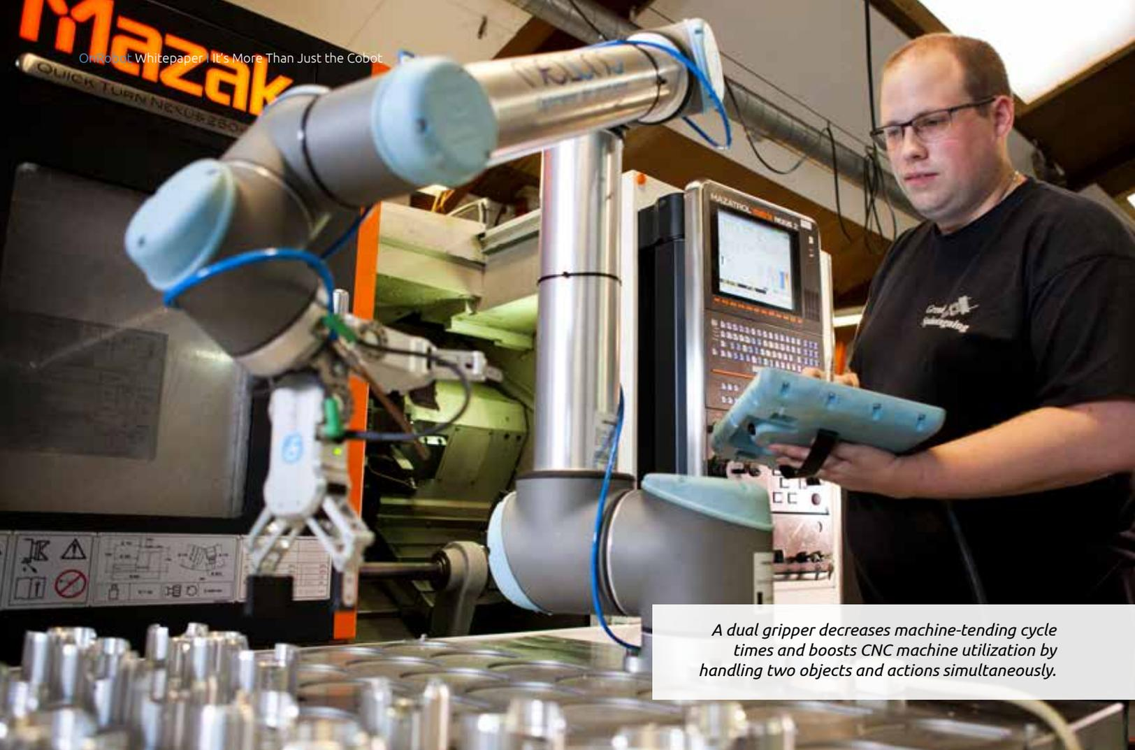
*A dual gripper decreases machine-tending cycle times and boosts CNC machine utilization by handling two objects and actions simultaneously.*
